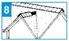
Ridge-to-roof application requires a mitre-cut to maintain continuous ridge line appearance.
